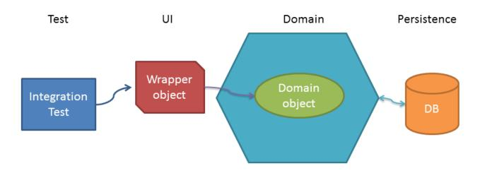
If the test invokes an action that is disabled, then the wrapper will throw an appropriate exception. If the action is ok to invoke, it delegates through.
