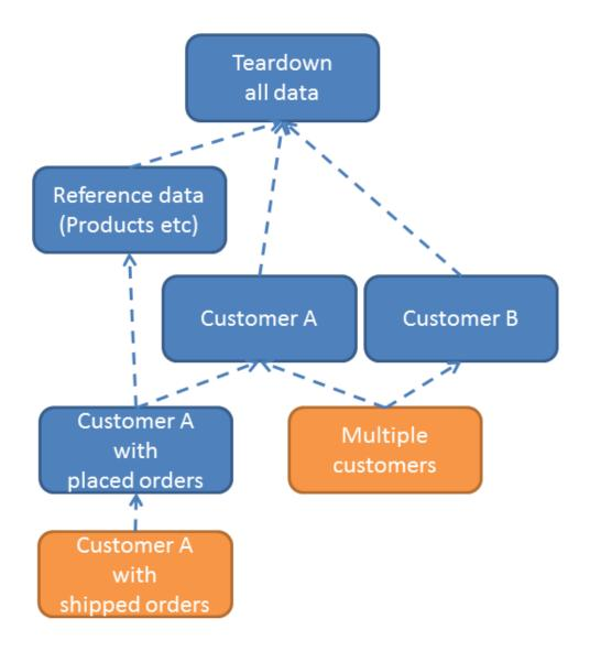
Back in the earlier section we noted the MultipleExecutionStrategy setting. We can now explain the meaning of this: the enum value of EXECUTE is designed for the flat style (where every fixture script will be called), whereas the enum value of IGNORE is designed for the composite style, and ensures that any fixture scripts visited more than once (eg TearDown) are only every executed the first time.
