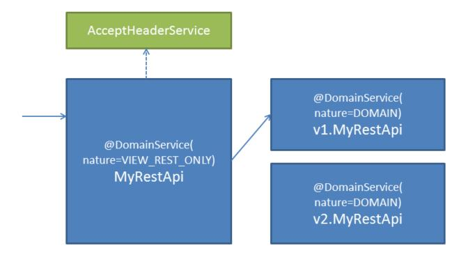
The REST request is submitted to a domain service with a nature of VIEW\_REST\_ONLY (MyRestApi in the diagram). This uses the AcceptHeaderService to obtain the values of the HTTP Accept header. Based on this it delegates to the appropriate underlying domain service (with a nature of DOMAIN so that they are not exposed in the REST API at all).
